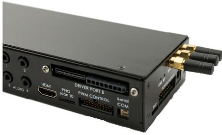
**Special Note:** There are 3 slots for antennas labeled W (for WiFi) C (for Cellular), B (for Bluetooth). The system ships standard with two antennas, these antennas should be attached to the W and B connectors (the two outside connectors) leaving C open.
